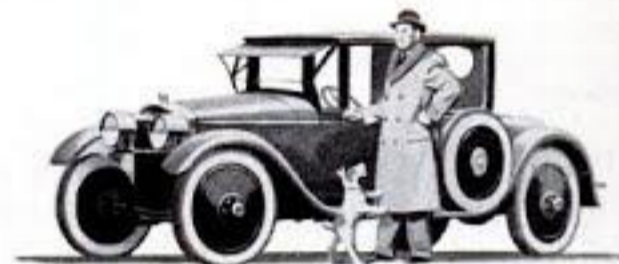
1922 JULIAN featured an airplane-type radial engine mounted on its side over the rear springs. The engine had six cylinders, developed sixty horsepower, and its backers claimed that it delivered twenty-five miles to the gallon.
